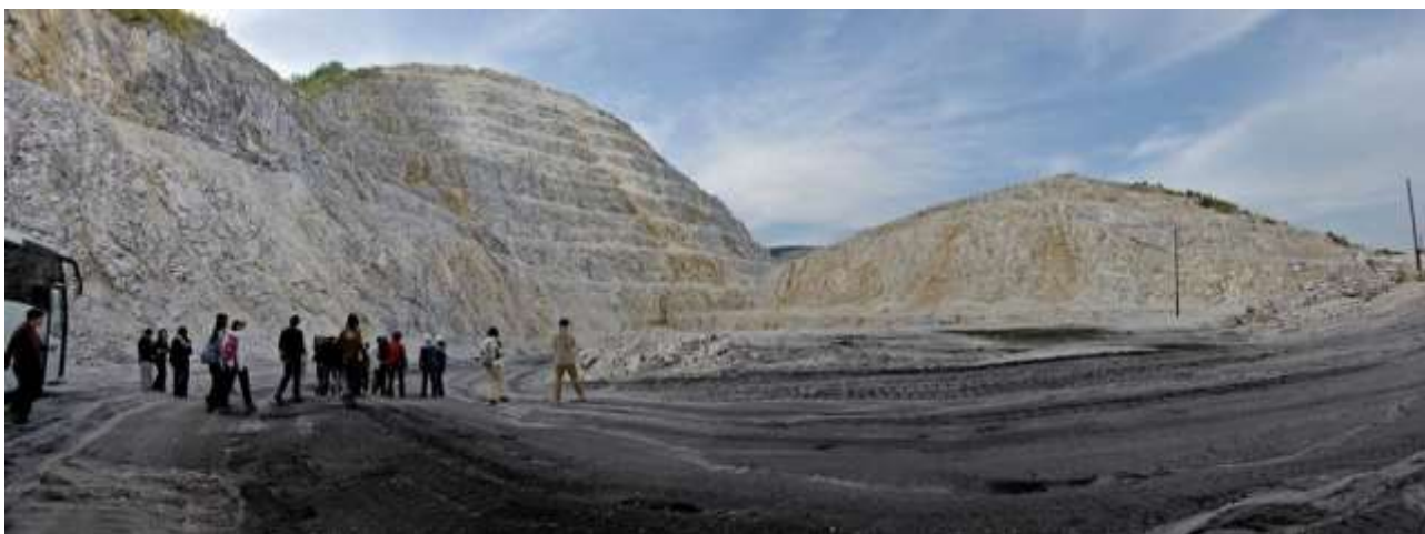
Fig. 3. Lower level of the Pereval quarry for the extraction of low-magnesia marbles for cement production, photo 0737-40.
